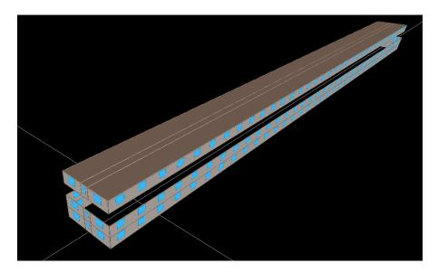
Note: The middle floors, since they thermally equivalent, are simulated as a single floor, and theresults are multiplied by 2 to represent the energy consumption of the 2 middle floors.
