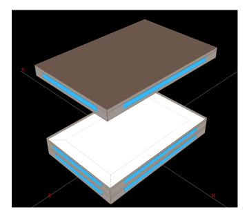
Note: The middle floors, since they thermally equivalent, are simulated as a single floor, and theresults are multiplied by 8 to represent the energy consumption of the eight middle floors.
